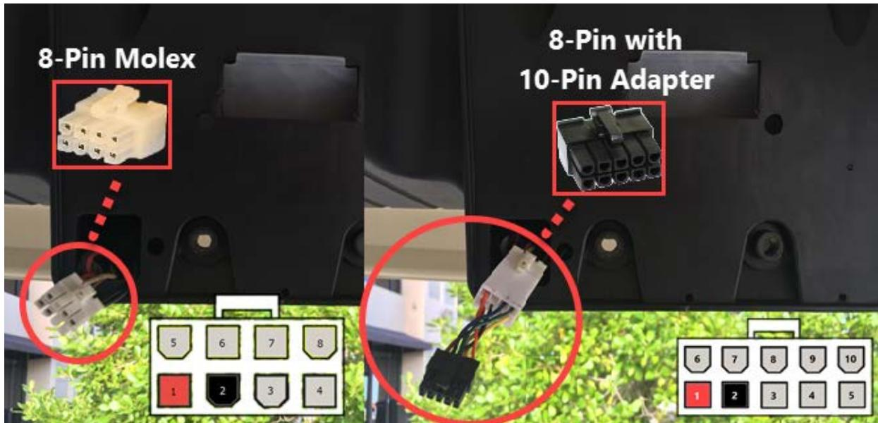
1. Use a number 2 or 3 Phillips hand driven screwdriver to remove the VDU from the console and expose the Molex connector.
