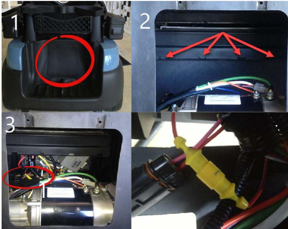
1. Remove the access cover located at the rear of the car.
