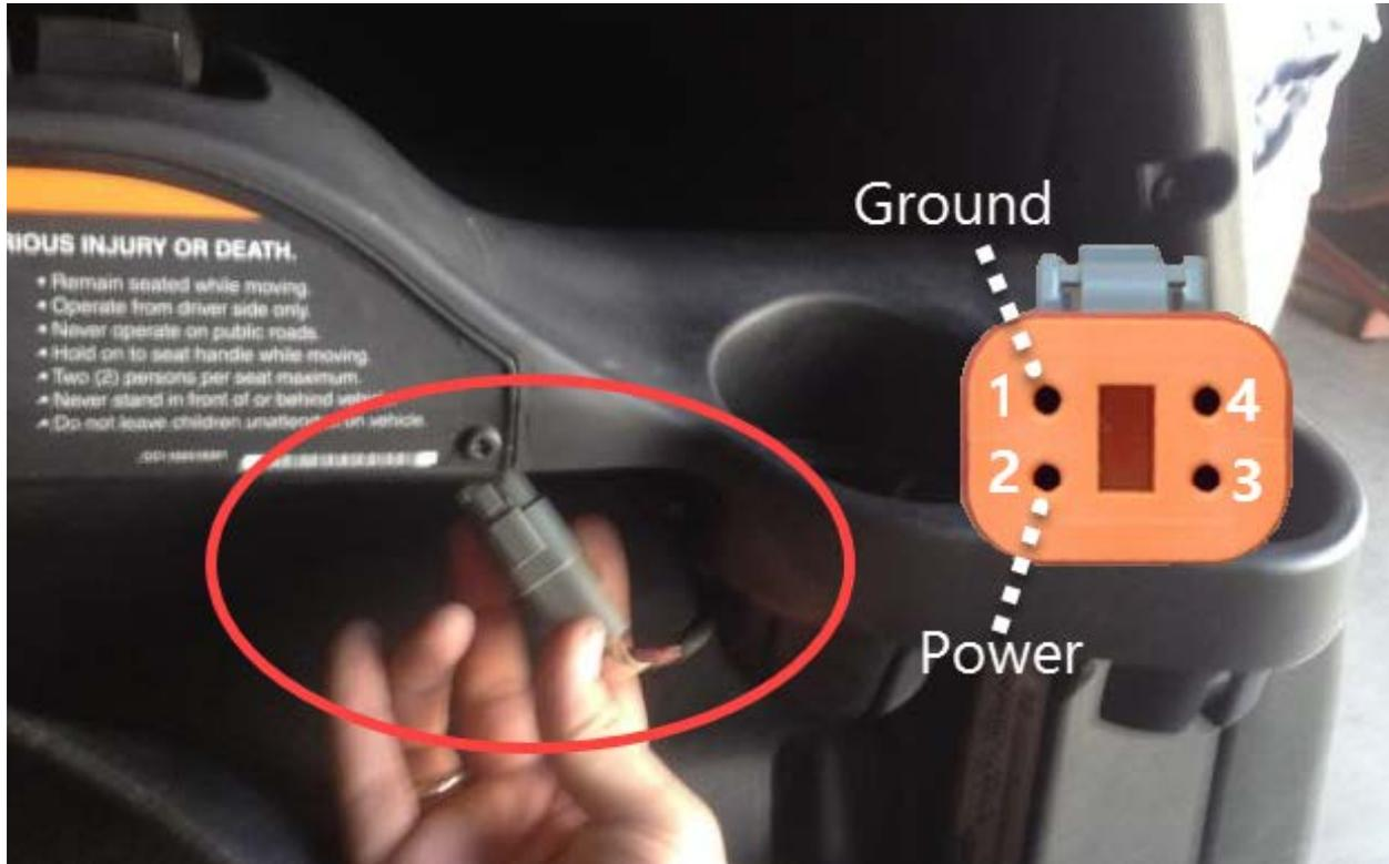
1. Pull the floor liner back on the passenger side and carefully pull down the harness that connects the passenger strut wiring to the motor controller.
